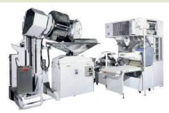
ECP proofer mounted in an automatic line for baguettes
