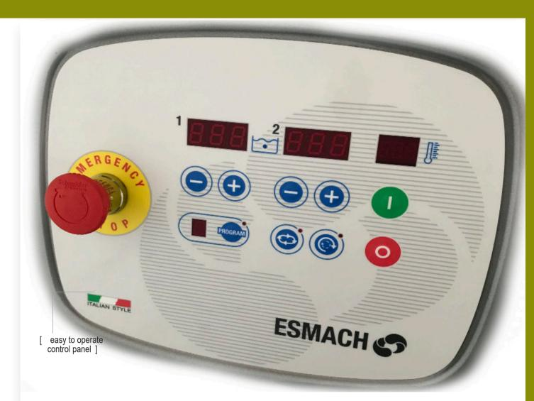
[ command push button on the machine side ]
