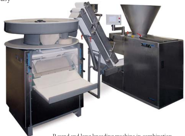
Round and long kneading machine in combination with a TA dough weigher, including high conveyor
