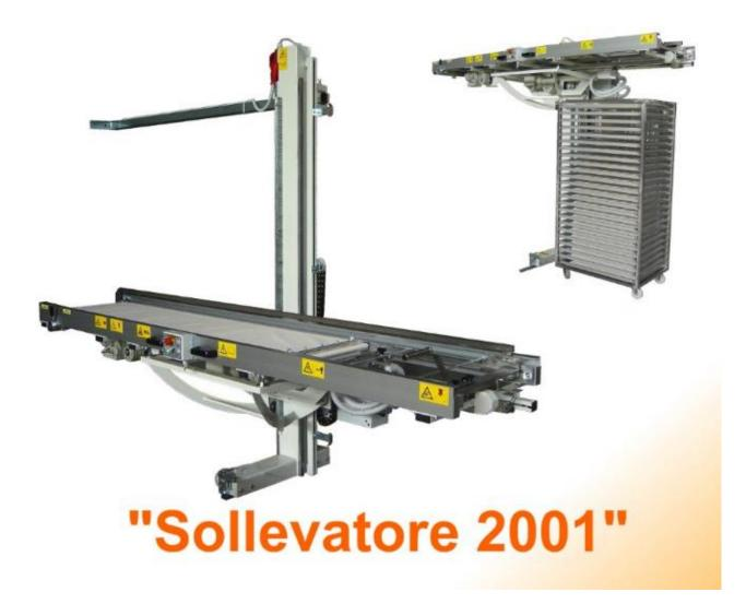
Loading and unloading with electric lifting for the deck positioning, electric entry and exit from the oven, manual belt recovery for the loading position. Max Width: 700 mm. Max depth: 2000 mm.
