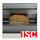
ISC® (Intelligent Slicing Control) (patent JAC) Automatic control system of pressure and slicing speed. It adapts the cutting action according to the consistency of the bread. no manual setting needed.
