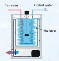
The ice water chillers are equipped with a digital **Ice Mass Sensor (IMS)** allowing optimum control over the accumulation of ice and maximum continuity. This also prevents the water spiral from freezing.
