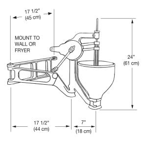
(NOTE: Diagram includes plunger, cylinder and mounting bracket purchased separately)
